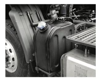
Our tanks use high-strength High Density Polyethylene (HDPE) or Linear Low Density Polyethylene (LLDPE). These materials are particularly dense and dimensionally stable. These engineering plastics are also longterm resistant to AdBlue® and other aggressive liquids from the automotive sector, are chemically very stable, resistant to abrasion and are characterized by high impact resistance. Our AdBlue® tanks are approved for AdBlue® according to DIN 70070 and ISO 22241/1.
