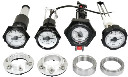
These displays are used for tanks without a power supply, as an additional tank display directly on the tank or for tank containers and interchangeable tanks. Application liquids: AdBlue®, oils, water and chemical and biological additives. Measuring ranges, lengths up to 800mm.
