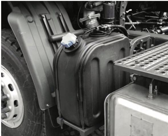
Our tanks use high-strength High Density Polyethylene (HDPE) or Linear Low Density Polyethylene (LLDPE). These materials are particularly dense and dimensionally stable. These engineering plastics are also long-term resistant to AdBlue® and other aggressive liquids from the automotive sector, are chemically very stable, resistant to abrasion and are characterized by high impact resistance. Our AdBlue® tanks are approved for AdBlue® according to DIN 70070 and ISO 22241/1.
